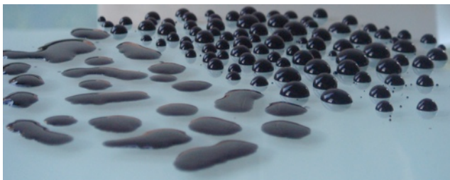
See the difference between the untreated and treated glass surface.
